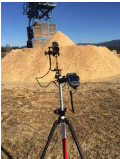
*Fig. 1: LTI's TruPulse 360 laser running MapSmart + Volume*
